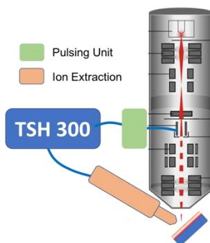
The **TSH 300** is easy to integrate into the HIM by just occupying **one single free port** of the chamber. No modifications of the HIMs ion column necessary leaving the imaging capabilities of the device untouched. Switching between standard secondary electron imaging and SIMS takes just a few seconds.
